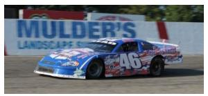
The LATE MODEL SPORTSMAN feature a great looking stock style template body similar to a NASCAR Monster Energy Cup car and are many tracks' top division. These cars race on 8" wheels and tires as opposed to the 10" wheels of an Outlaw Super Late Model and can run on either a stock or fabricated chassis. Expect lap times in the 13-14 second range (96-104 MPH). The cost to build a car is in the \$25-30,000 range.
