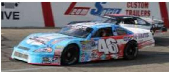
The **LATE MODEL SPORTSMAN** feature a great looking stock style template body similar to a NASCAR Monster Energy Cup car and are many tracks' top division. These cars race on 8" wheels and tires as opposed to the 10" wheels of an Outlaw Super Late Model and can run on either a stock or fabricated chassis. Expect lap times in the 13-14 second range (96-104 MPH). The cost to build a car is in the \$25-30,000 range.
