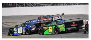
The Outlaw Super Late Models are Kalamazoo Speedway's premier division. These outlaw-bodied racecars have a full tubular frame, quick change rear ends and coil over suspension. Their engines are a cast iron block, but that's about the only original equipment on the drive train of one of these fast cars. You'll find the best of the best drivers coming from a tristate area. This division runs several races of 100 laps and more and are the stars of three of the Speedway's marquee events: The
