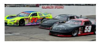
The Super Stocks feature a great looking stock style template body similar to a NASCAR Monster Energy Cup car you'd see on TV. These cars race on 8" wheels and tires as opposed to the 10" wheels of an Outlaw Super Late Model and can run on either a stock or fabricated chassis. The Super Stocks are many tracks' top division. Expect lap times in the 13-14 second range (97-104 MPH). The cost to build a car is in the \$25-30,000 range.
